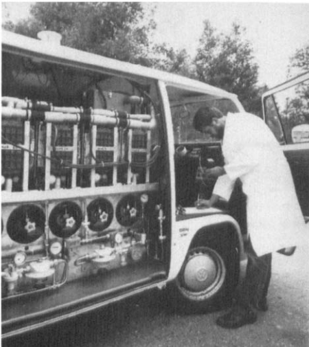
Fig. 2. Testing of fuel cell stacks in an electric van.
